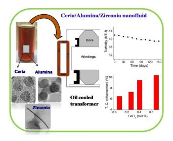
Transformer oil (TO) based nanofluids containing either ceria nanocubes (0.08–0.7 vol%), zirconia nanorods (0.03–1.7 vol%), and alumina nanospheres (0.02–0.2 vol%), were prepared via a two-step method. The thermal decomposition of their respective oleate precursor in a high boiling solvent was used for the fabrication of oil dispersible
