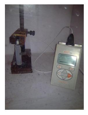
**Fig. 2** Optical photograph of a KD2 Pro thermal conductivity meter in which a platinum hot wire is immersed in the nanofluid which acts as both the heater and temperature sensor.
