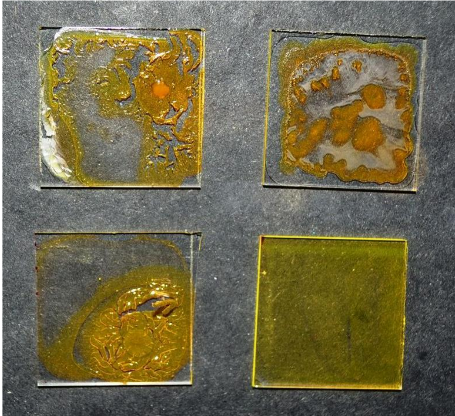
Figure 5.4: Photograph of bilayer DNA-PG film (top left) and bilayer DC-PG film (top right) prepared by immersion technique; DNA:PG (bottom left); and DC:PG film (bottom right) prepared by drop casting technique.
