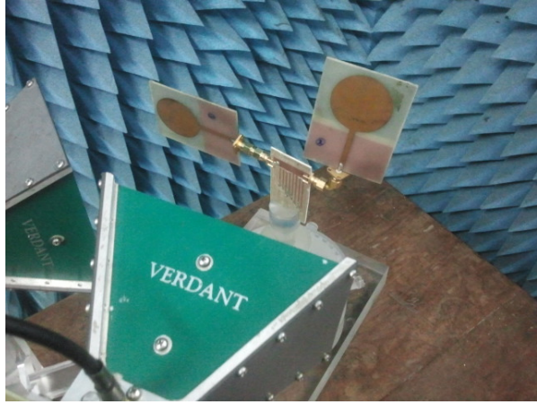
Fig. 3.13: Experimental setup for bistatic measurement of the RFID tag using shorted stub multiresonator
