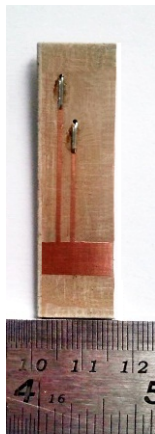
Fig. 3.27: Photograph of fabricated multiresonator with two shorted stubs
