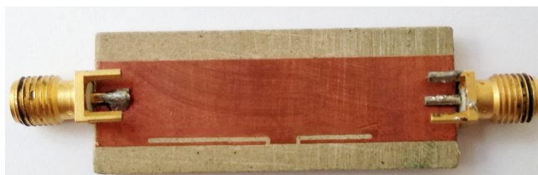
Fig. 4.30: Photograph of fabricated multiresonator with two spurlines
