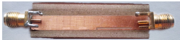
Fig. 4.25: Photograph of fabricated spurline resonator
