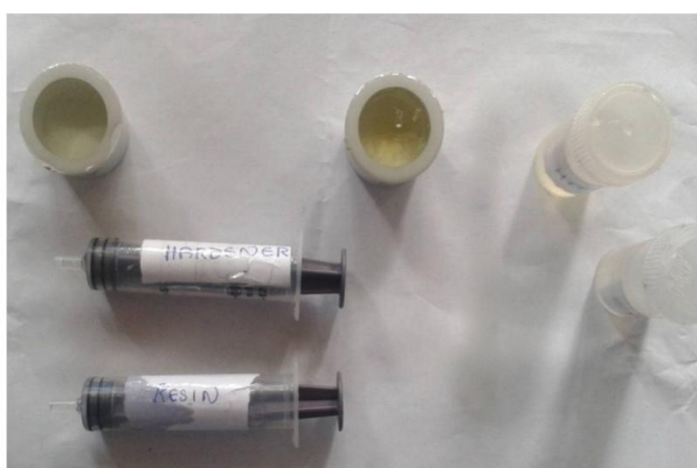
Figure 7.3: Epoxy and Hardener in syringes. Various blends of hardener and epoxy as per table in 10ml containers
