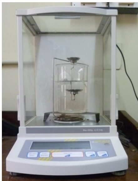
Figure 3.22 Balance with Density measurement kit
