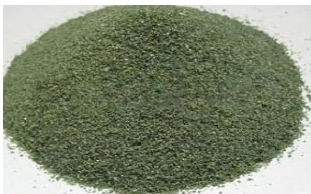
Figure 3.1: Photograph of SiC particles of average particle size of 23 \mu\text{m}
