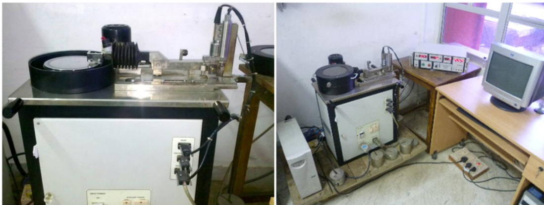
Figure 3.16: DUCOM (TR-20 LE) pin on disc tribometer with the computer interface
