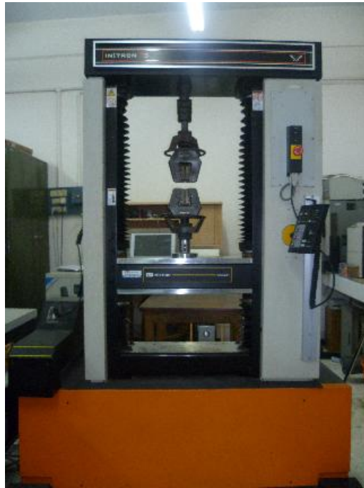
Figure 3.12: INSTRON 1195 - 5500R series electromechanical materials tester
