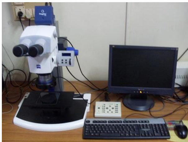
Figure 3.19: Photograph of Prog Res C5 stereo microscope
