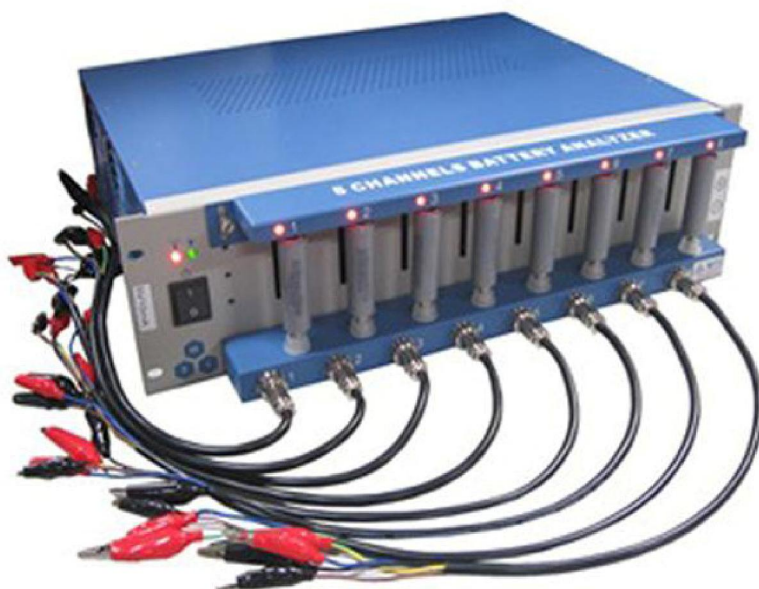
Figure 8: The eight channel GCD set up (MTI Corporation)
