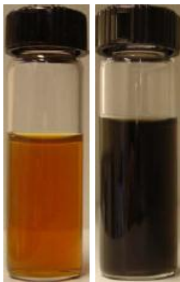
Figure 3.8: (a) Graphene oxide dispersed in water, (b) Reduced graphene oxide dispersed in DMF
