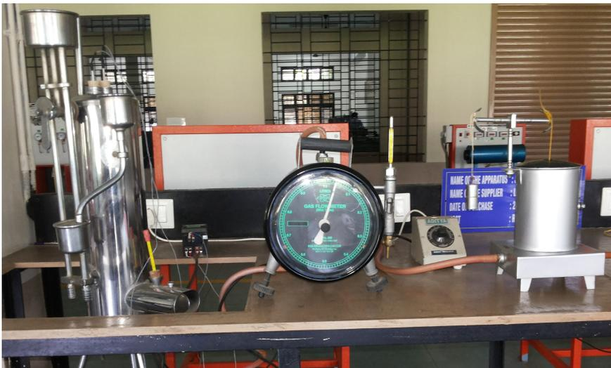
Figure 6.2: Junkers gas calorimeter apparatus
