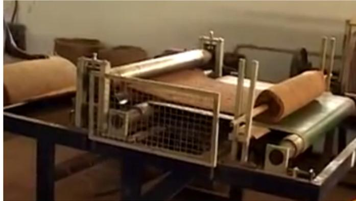
Figure 3.5: Glue Spreading Machine
