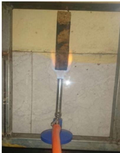
Figure 6.8: Rate of burning test apparatus
