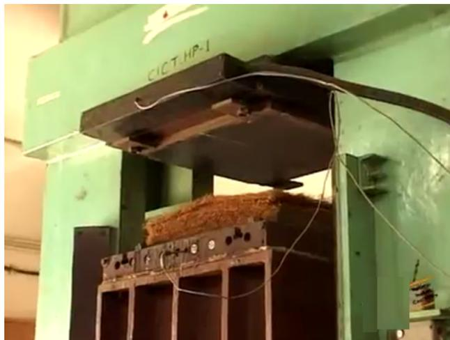
Figure 3.6: Hydraulic Hot Press
