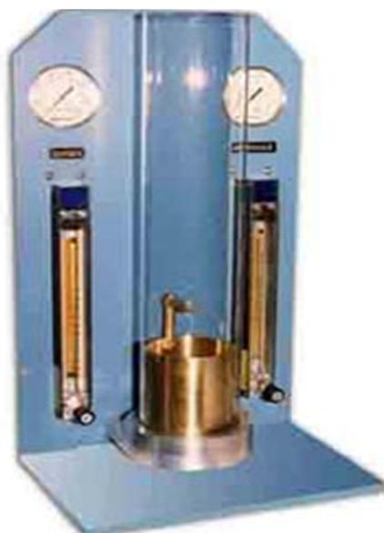
Figure 6.1: Limiting Oxygen Index Tester
