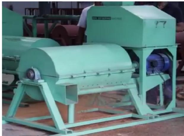
Figure 3.3: Mobile Fibre Extraction Machine
