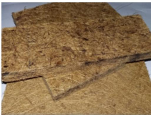
Figure 3.2: Medium density fibre boards manufactured from coir
