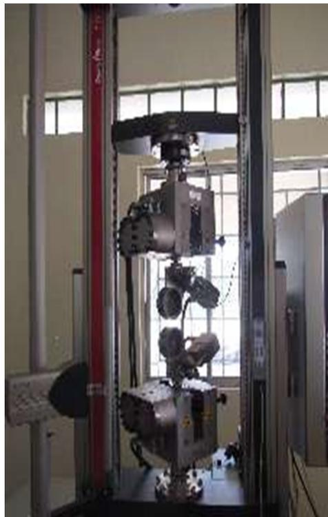
Figure 5.2: Universal Testing Machine for measuring tensile, bending and compressive properties of coir fibre boards
