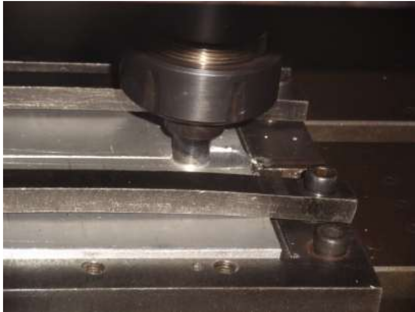
Fig. 1.4. FSW in progress
