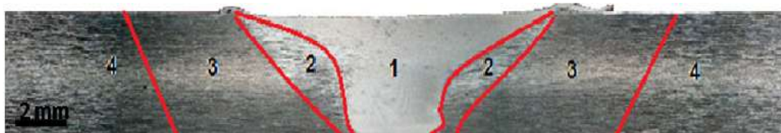
Fig.1.3 : Macroscopic regions of friction stir weld.
