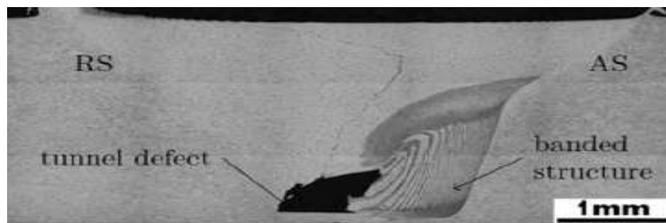
Fig.2.9. Worm hole or tunnel defect [69]
