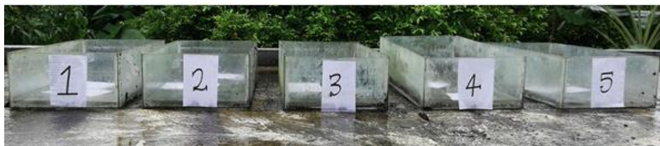
Figure 6.34: Experimental set up for comparing the degradation of plastics in different types of water.
