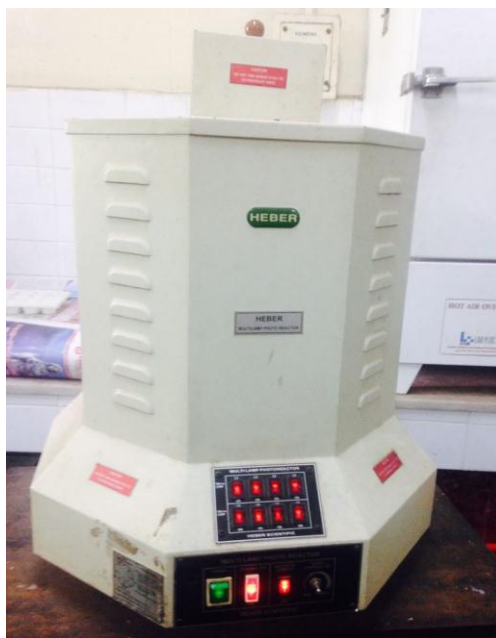
Figure 4.11: Multilamp photoreactor-external view
