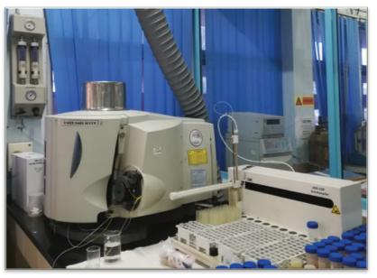
Fig. 6.3 Inductivity Coupled Plasma–Optical Emission Spectrometer
