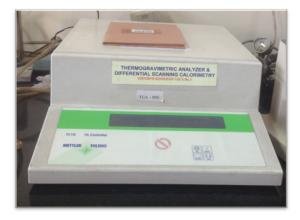
Fig. 8.3 Differential scanning colorimeter
