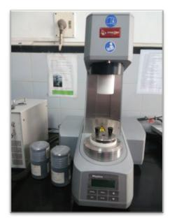
Fig. 7.4 Controlled-Stress Rheometer
