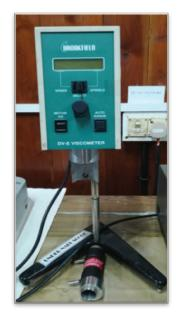
Fig. 7.5 Viscometer
