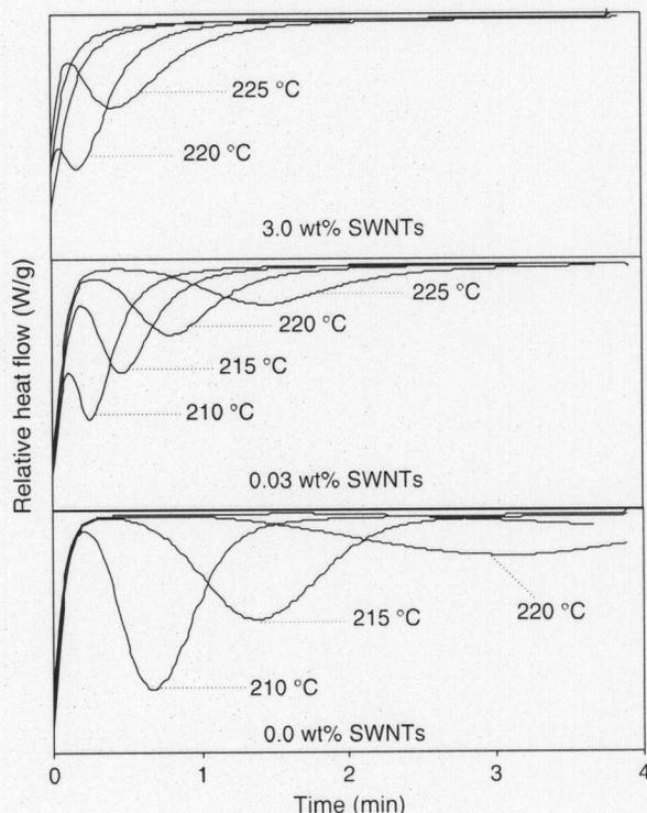
Fig. 2. Heat flow during isothermal crystallization of PET-SWNT nanocomposite samples.
