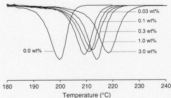
Fig. 1. DSC cooling scans (20 °C/min from 310 °C melt) of PET-SWNT nanocomposite samples.
