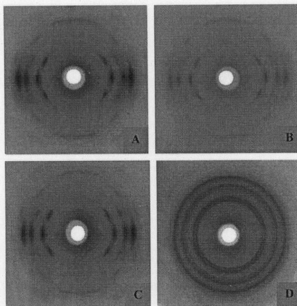
Fig. 4. WAXD patterns of the following samples: (A) PET/SWNT 1 wt% nanocomposite film after drawing, (B) PET/SWNT 1 wt% nanocomposite film after melting and subsequent slow cooling at constant length, (C) neat PET film after drawing, (D) neat PET film after melting and subsequent slow cooling at constant length. The drawing direction was vertical.
