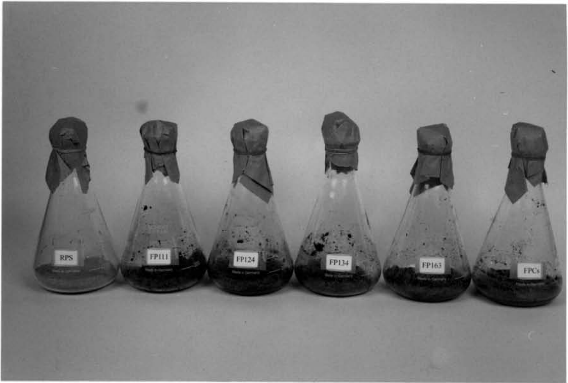
Fig 6.1 Fermentation of prawn shell waste being carried out in Erlenmeyer flasks under laboratory conditions
