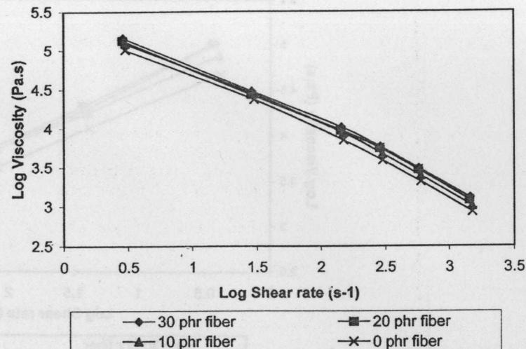
FIGURE 1 Shear viscosity versus shear rate at 80°C.
