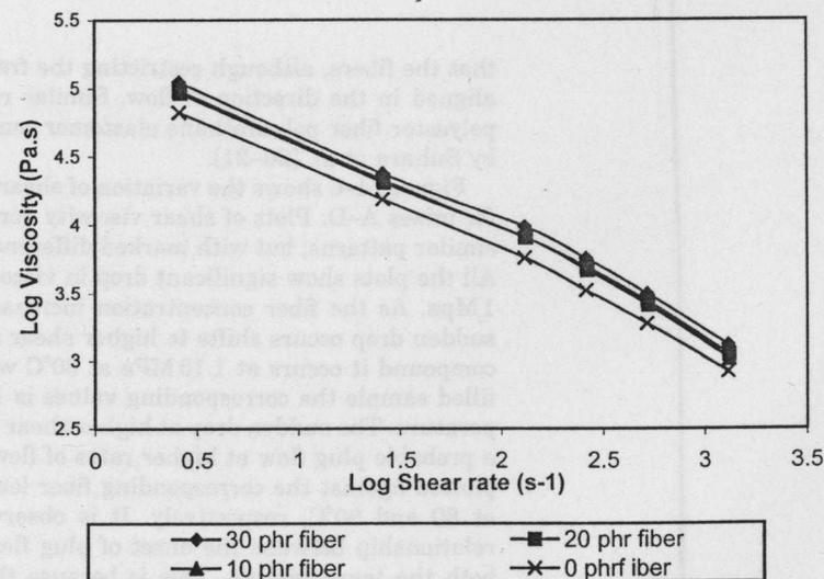
FIGURE 2 Shear viscosity versus shear rate at 90°C.
