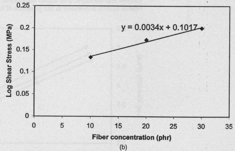
FIGURE 7 a) Variation of shear stress at the point of inflection with fiber loading at 80°C. b) Variation of shear stress at the point of inflection with fiber loading at 90°C.
