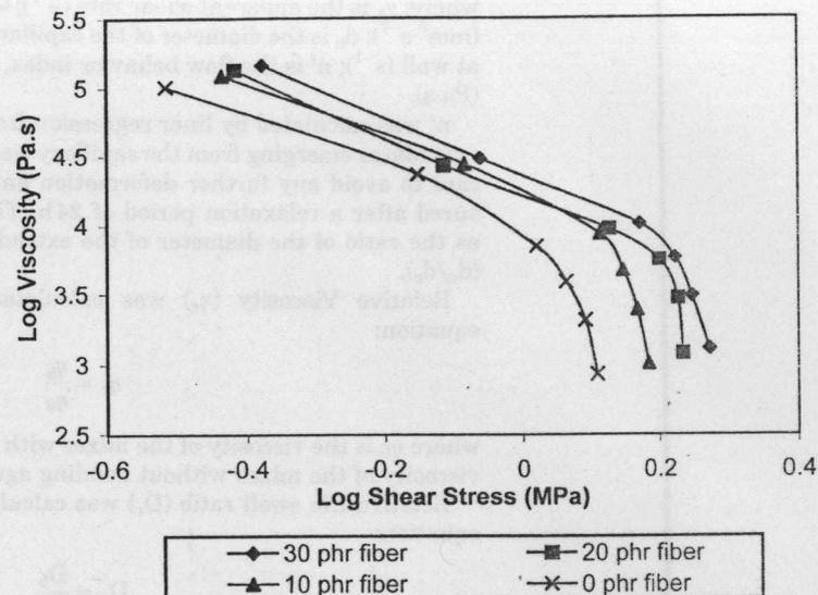
FIGURE 4 Shear viscosity versus shear stress at 80°C.
