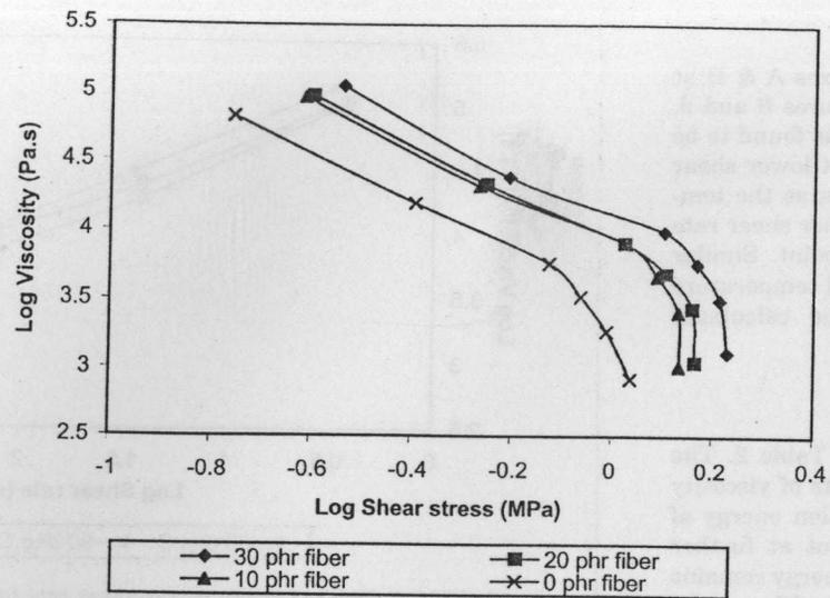
FIGURE 5 Shear viscosity versus shear stress at 90°C.
