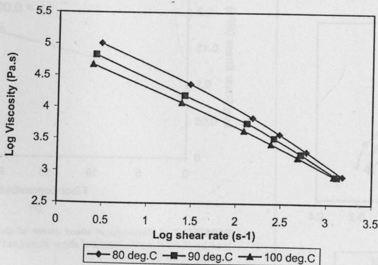
FIGURE 8 Shear viscosity versus shear rate for Mix A.
