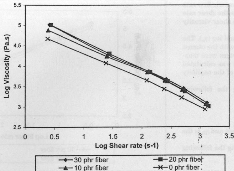
FIGURE 3 Shear viscosity versus shear rate at 100°C.
