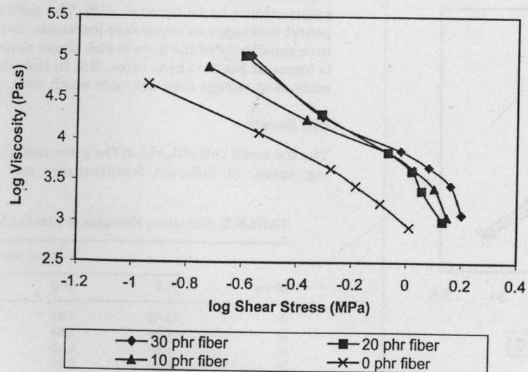
FIGURE 6 Shear viscosity versus shear stress at 100°C.
